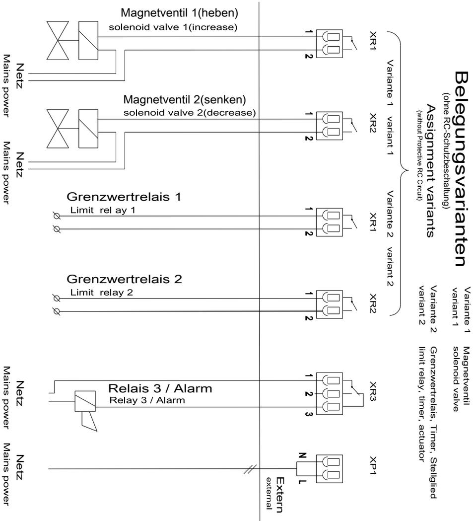
Fig. 19: Terminal diagram with assignment options 1
