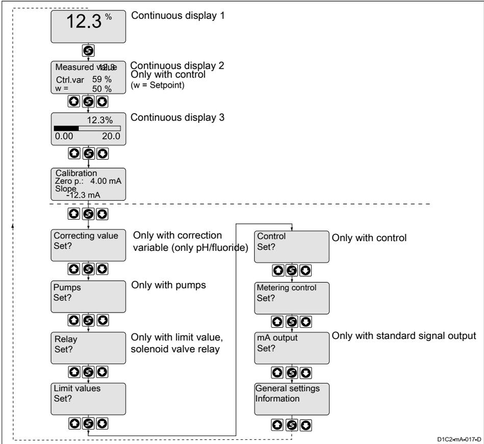
Fig. 50: Complete operating menu / Shown with measured variable % and the measuring range 0%.... 100%
