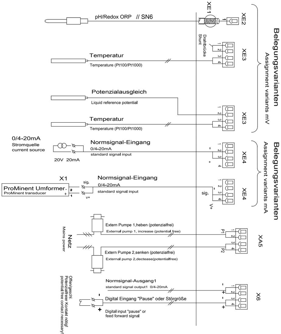
Fig. 20: Terminal diagram with assignment options 2
