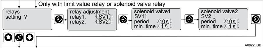
Fig. 59: Solenoid valve relay
