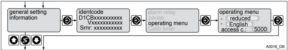
Fig. 70: Device configuration
