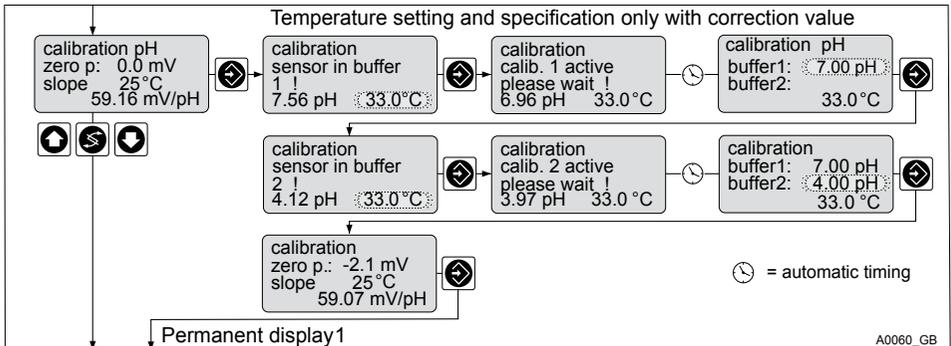
Fig. 43: Calibration of pH sensors
