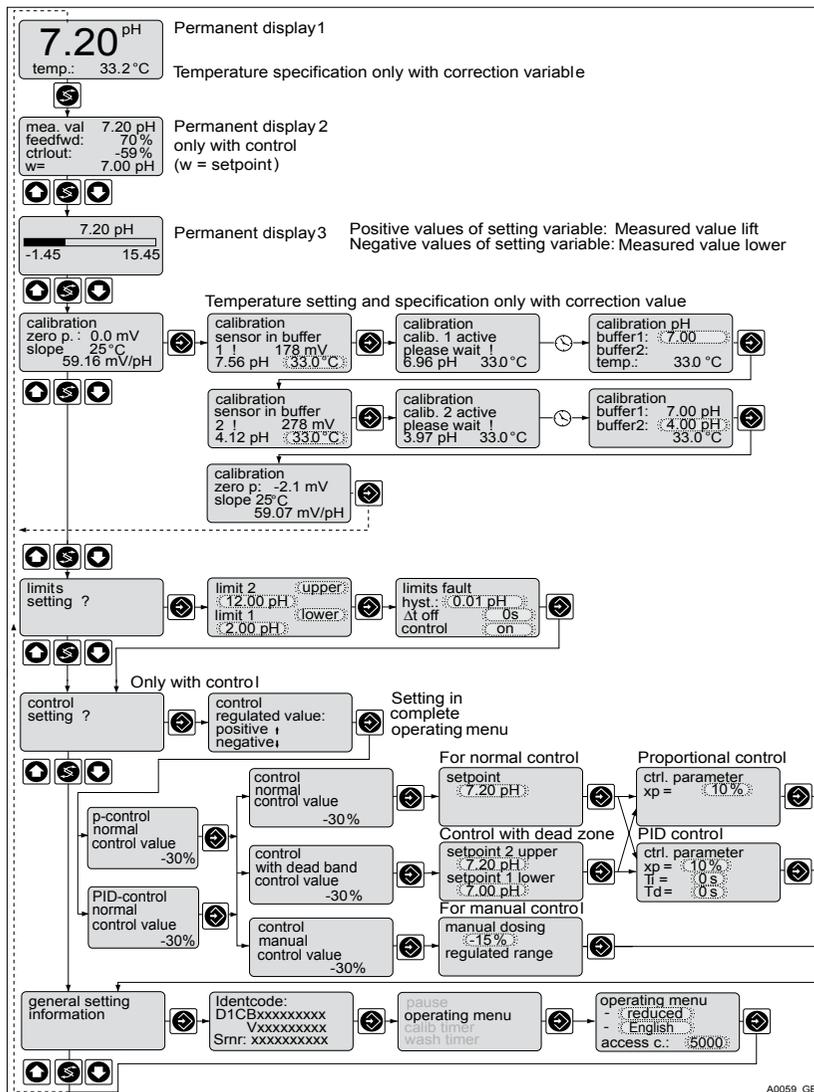
Fig. 41: Reduced pH / redox / fluoride operating menu (shown with the example of pH)
