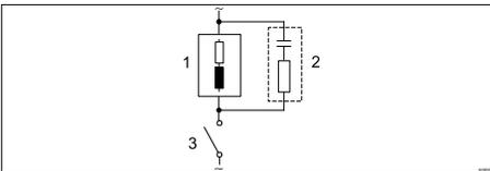
*Fig. 15: RC protective circuit for the relay contacts*
