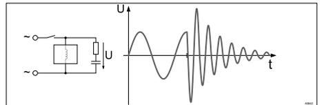
*Fig. 21: Switching-off process shown on the oscillogram.*
