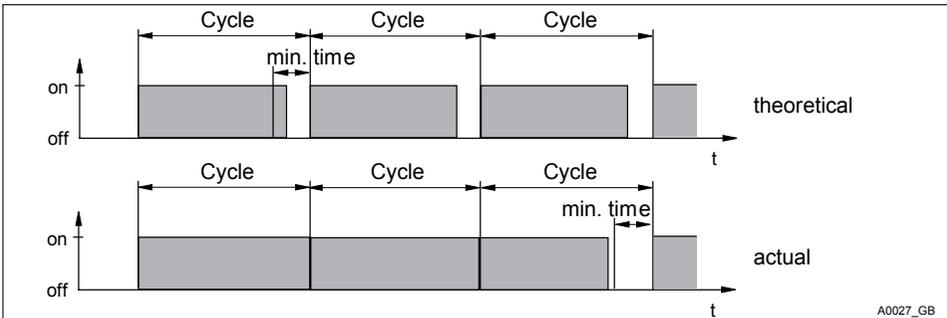
Fig. 62: Theoretical switching time > (cycle - min. time) and calculated switching time < cycle
