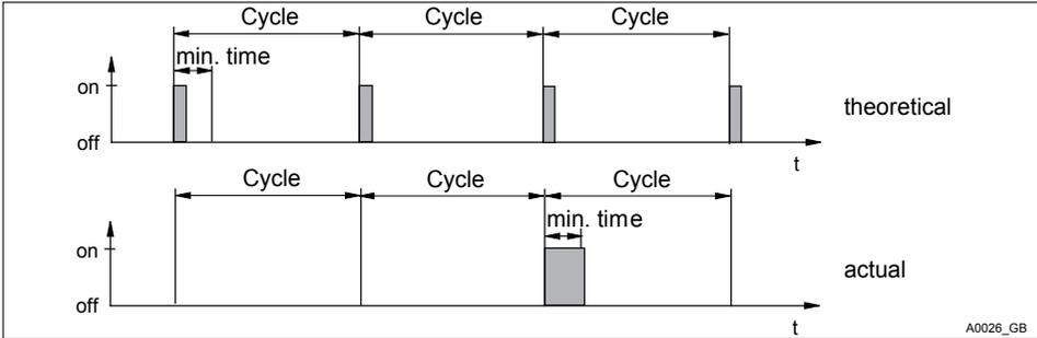
Fig. 61: Theoretical switching time < min. time
