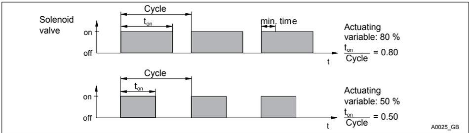
Fig. 60: Solenoid valves
