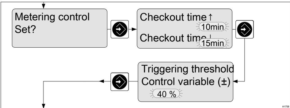
Fig. 66: Metering time: Adjusting the checkout time and control variable triggering threshold.
