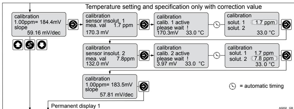
Fig. 45: Calibrating the fluoride sensor
