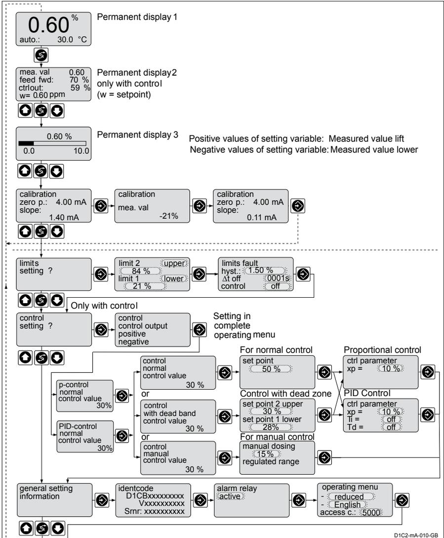
Fig. 49: Reduced operating menu / Shown with measured variable % and the measuring range 0%....100%
