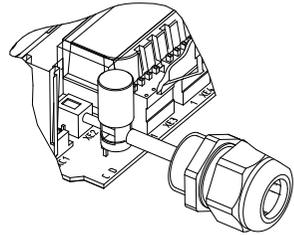
Fig. 9: Preparation of coaxial cable
