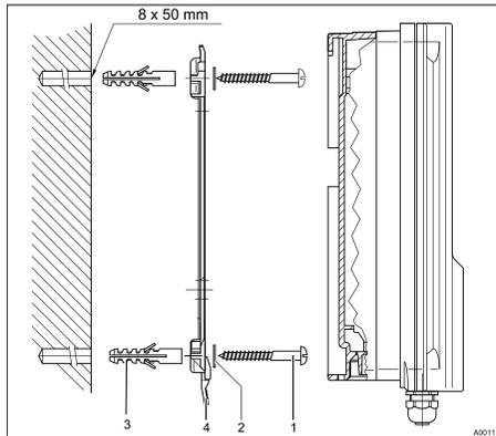
Fig. 3: Fixing material for wall mounting
