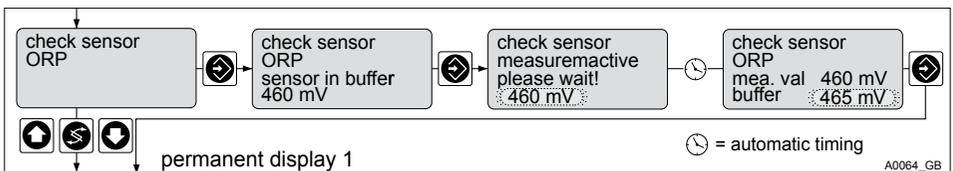
Fig. 44: Testing redox sensors
