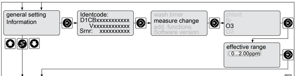
Fig. 24: Selection of measured variable and measuring range
