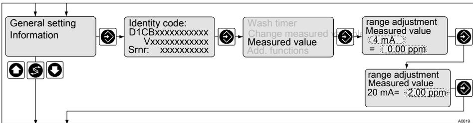
Fig. 72: Setting the measured value (for example "chlorine")
