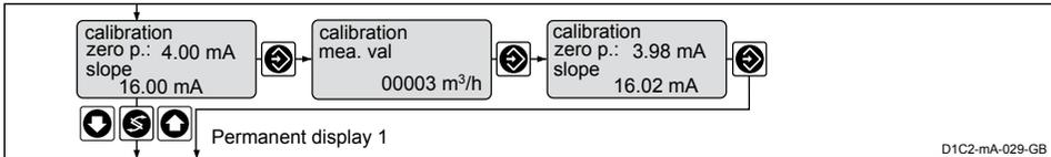
Fig. 51: Zero point calibration menu / shown with flow as the measured variable and the measuring range 0... 100 m<sup>3</sup>/h
