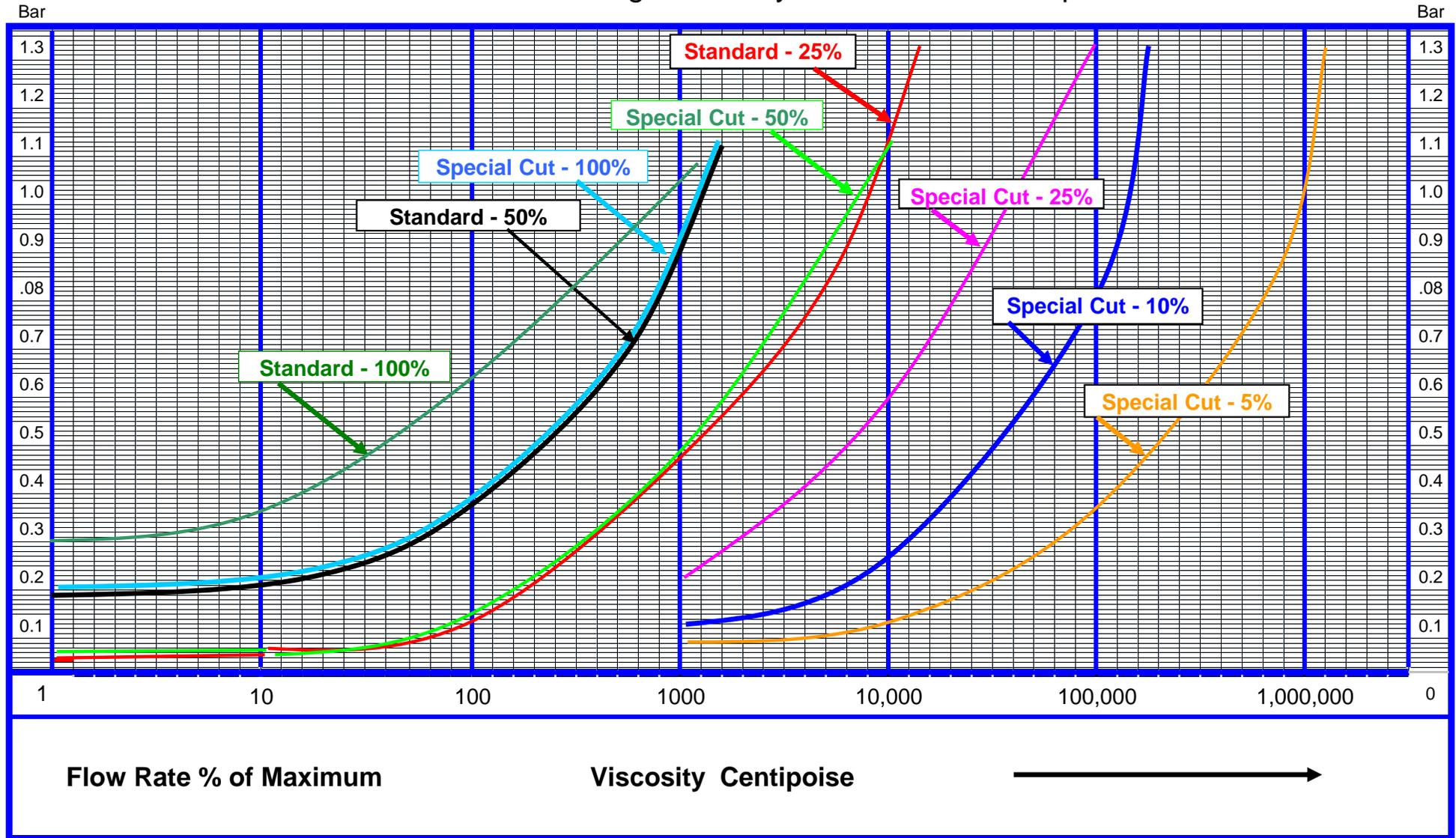
This graph is intended as an aid to determine the pressure drop of the measuring device as part of a system, allowing engineers to calculate the most economic components for their systems, i.e. pump selection would be determined on the total system pressure drop, the lower the pressure drop the lower the cost of the pumping component.
