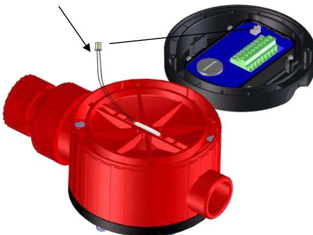
Remove the 4 Torx screws (torque max. 0.5 Nm)
