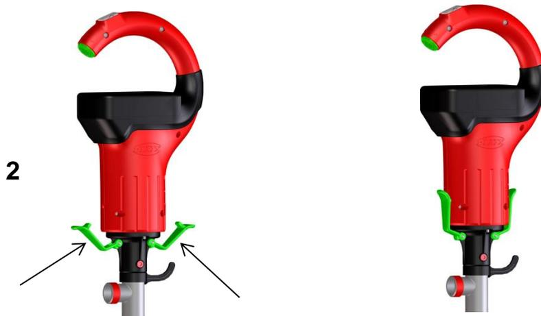
Press the clamping levers towards the motor until they are both audibly locked. To remove the motor unlock the two clamping levers.
