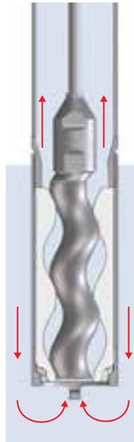
The pump works on the displacement principle. Its worm-shaped impellor (eccentric worm) is guided in a stator shaped as a mating counterpart. This creates closed cavities during rotation in which the fluid is transferred upward continuously in an especially gentle manner and almost without pulsation.
